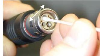
Select the dry cotton bud and using one end of it, apply to the ferrule face and gently wipe across it. This will thoroughly dry the ferrule. Use a cotton bud end once only as they quickly become contaminated.
