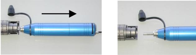
Unscrew the endcap from the tool, and remove a new cotton bud
