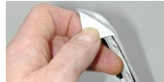
Clean the ceramic ferrule by applying the alcohol damped end of the cotton bud to the ferrule end face and gently wiping it across the endface.
