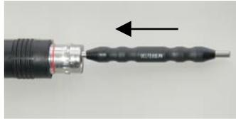
If, after successfully cleaning and inspecting all ferrules, the system still exhibits high insertion loss this may be due to a damaged or contaminated alignment sleeve. Try replacing this part (LEMO Part no PSS.F2.290.NZZ) and check the system again.
