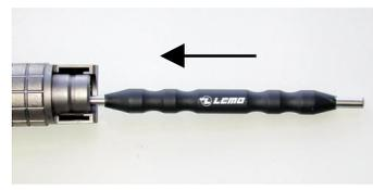
If, after successfully cleaning and inspecting all ferrules, the system still exhibits high insertion loss this may be due to a damaged or contaminated alignment sleeve. Try replacing this part (LEMO Part no PSS.F2.290.NZZ) and check the system again.
