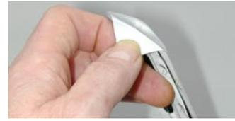
Clean the ceramic ferrule by applying the alcohol damped end of the cotton bud to the ferrule end face and gently wiping it across the endface.
